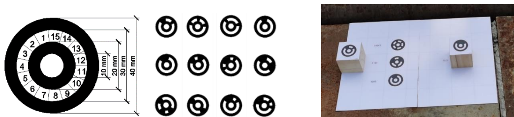
Fig. 3. Marker points (left) and benchmark plate (right)
