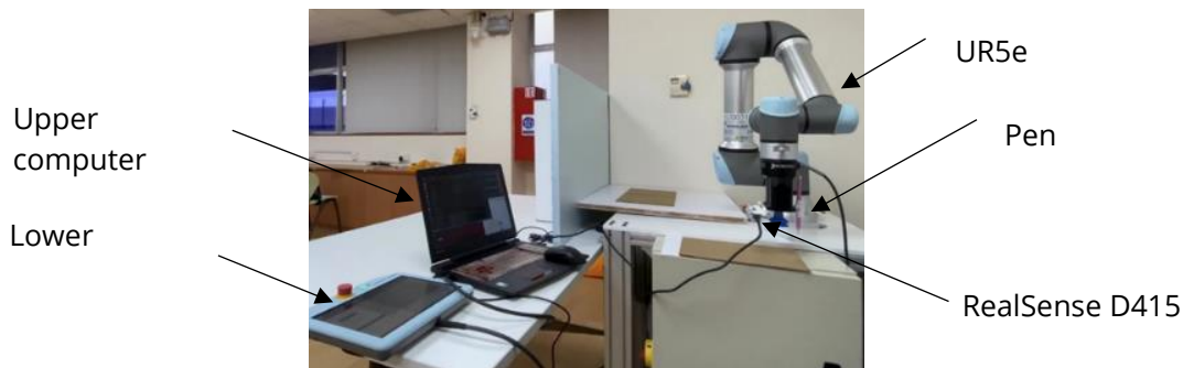
Fig. 1. Hardware configuration of the platform
